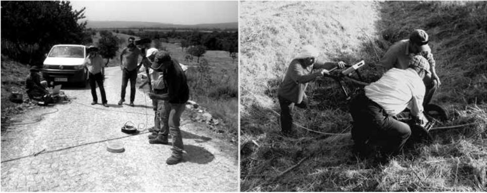
Fig. 1. Refraction seismic fieldwork (left) and GPR fieldwork (right) in Ephesos
