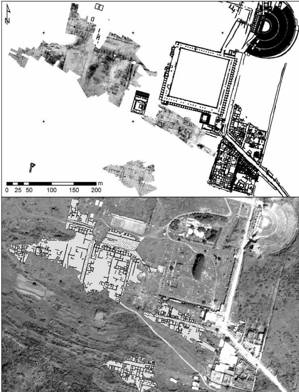
Fig. 3. The results of GPR prospection in the area of the Serapeion in Ephesos above (black: high amplitudes – reflective, white: low amplitudes – absorbent) and the archaeological interpretation below
